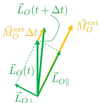
$$\vec{L}_O = \vec{L}_{O\perp} + \vec{L}_{O\parallel} \quad , \quad \vec{L}_{O\perp} \perp \vec{M}_O^{\text{ext}} \quad , \quad \vec{L}_{O\parallel} \parallel \vec{M}_O^{\text{ext}}$$
