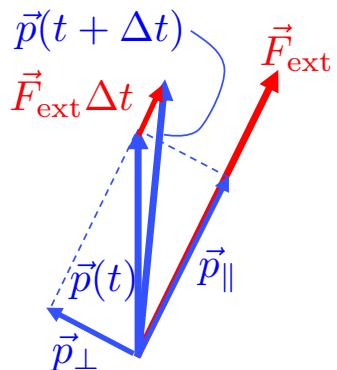
$$\vec{p} = \vec{p}_{\perp} + \vec{p}_{\parallel} \quad , \quad \vec{p}_{\perp} \perp \vec{F}^{\text{ext}} \quad , \quad \vec{p}_{\parallel} \parallel \vec{F}^{\text{ext}}$$
